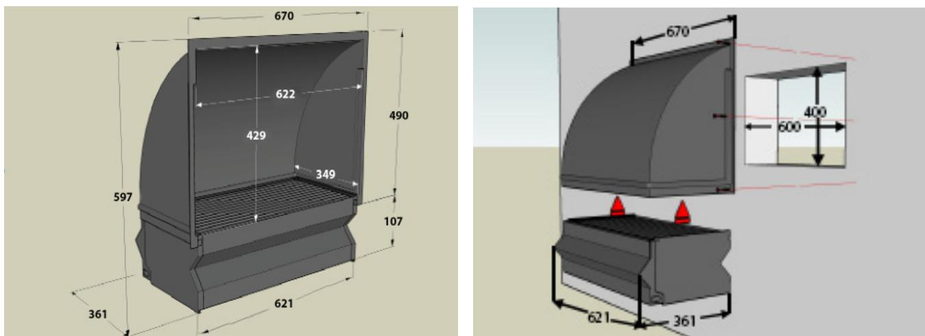
These are standard sizes in mm. Covers can be placed directly next to each other, and therefore are suitable for any type of air inlet.
