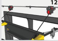
Mount 2 rollers above inlet and connect ropes with cable clamb to a rod
