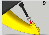
Place the fine tune screw and bolt
