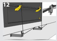
Mount 2 supports and connect ropes with cable clamb to a rod
