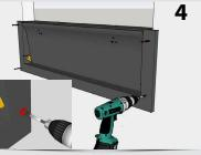
Mount bottom inlet into the hole with screws. Use pan head screw 5x60 with a flat washer
