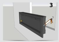
Put glue behind the flange of the firsth inletthis is the bottom inlet
