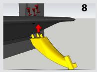
Screw ropeholder on the flap of the inlet with 3 screws
